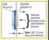
\*Note: Maximum recommended panel thickness is 0.062" (0.2cm). Dimensions in excess of 0.062" (0.2cm) can limit proper cable mating due to hex nut protrusion. Panels exceeding 0.062" (0.2cm) can be milled down to the recommended thickness in the area around the adapter.
