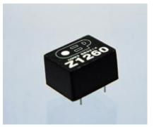
Provides isolation between modems or similar devices and telephone lines. This transformer is designed for use in voice or data transmission circuits where the line d.c. is diverted from the windings by a choke or solid state device. The use of this transformer should enable the equiptment it is used with to cpmly with the relevent requirments of BS6305.
