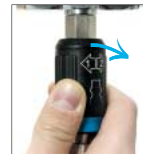
rotation in direction of the arrow disconnection of body and probe.
