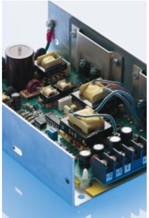
The application above uses punches parts to insulate the transistors from the mounting bracket and a sheet of Sil-Pad to isolate the mounting brackets from the frame of the assembly.
