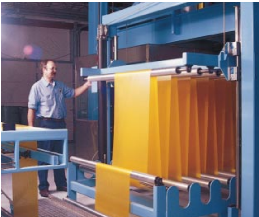
At Bergquist's Cannon Falls, MN manufacturing facility, a Sil-Pad material runs through a 3-story coating press.
