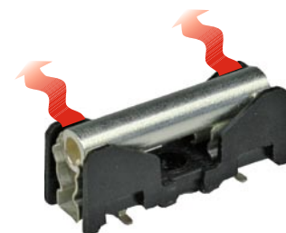
Fig. 5: UL/CSA test with silver tube
