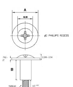
A one piece-fixing bolt can replace a three-part assembly of screw, washer and tube. Designed to give optimum Compression to the GVD range of dampers. The threads are suitable for screwing directly into a HDD. Available in UNC 6-32 or M3 thread.
