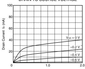
Drain to Source Voltage VDS (V)
