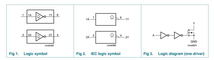
Low-power dual inverter with open-drain output
