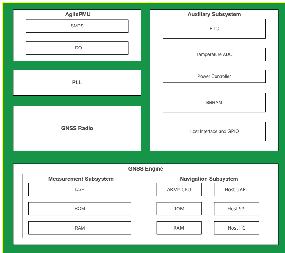
FIGURE 2 – SiRFstarV™ 5e GNSS SoC BLOCK DIAGRAM
