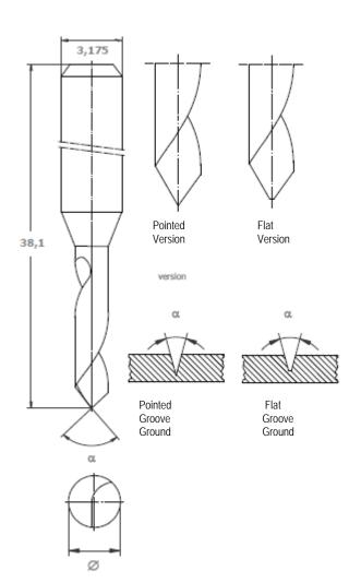
V-groove cutter made of carbide with one spiral twisted cut. Applications:
