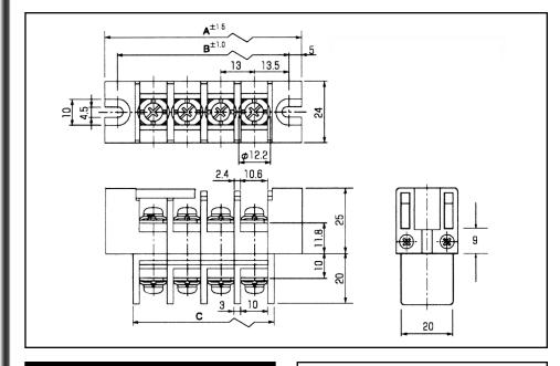
BlockMaster Electronics' new OTB-330N Series are medium-power, thru-panel terminal blocks available in 2-15 positions.
