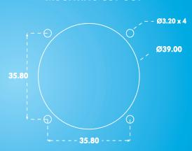
The joystick is dropped into the panel cut-out. For panel thickness of <3mm, M3 x 16 countersunk machine screws are recommended. Illustration (left) shows the square bezel option, a circular bezel is also available.
