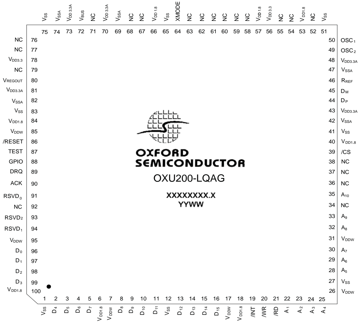
Figure 2 OXU200 100-Pin LQFP Package (Top View)
