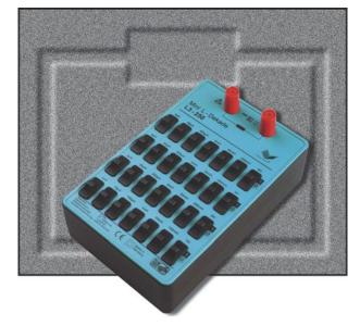
The L3-250 renders inductance values in a range of 7 decades:  $1 \mu H - 11,11111 H$ . A staggering of the inductance values in 1-2-3-4 steps allows an airtight adjustment by means of sliding switches. The tapped value equals the sum of the adjusted inductance values. The use of ferrite cores allows all these features to be included in one compact design. The supply is through 4 mm safety sockets.
