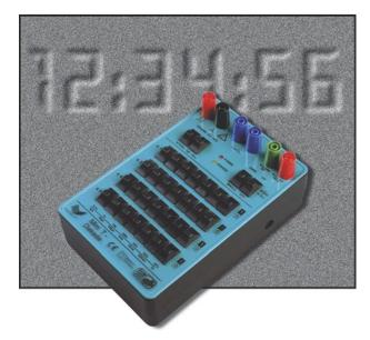
The Mini-T is a compact electronic precision timer (rectangle signals) independent from a power system. The adjustable range for the period is 1  $\mu$ s to >10 s and 0,1 s to >1 Ms (quartz stable). The period adjustment is by means of sliding switches in 1-2-4-8 steps (dual code). Apart from the continuous output signal the Mini-T offers the possibility of external triggering or gating. There are several outputs.
