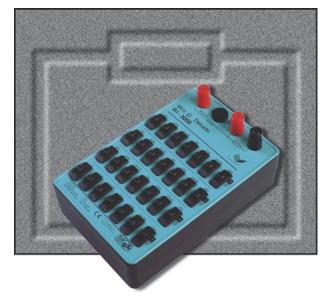
The R1-3000 compared to the R1-1000 offers a higher maximum power rating of 3 W. Additionally, the decade can be protected from an overload by using a quick-acting fine-wire fuse (a 400 mA fuse is supplied as standard accessory). By a non-fused resistance tap the internal resistance of the fuse can be by-passed. This ensures accuracy, particularly when low resistance values are concerned.
