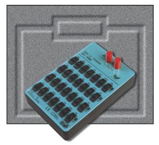
The R1-1000 is equipped with 28 joined 1 Ohm resistances which may be activated singularly by means of sliding switches. The staggering of the resistance values in 1-2-3-4 steps allows an airtight adjustment of the resistance values in 7 decades (1 Ohm to 1,11111 MOhm). The adjustment of 156 kOhm e.g. is made by choosing the following switches:100 kOhm, 40 kOhm + 10 kOhm, 4 kOhm + 2 kOhm.
