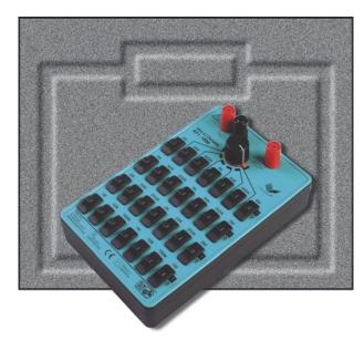
The RT1-1000 has the same technical features as the R1-1000. However, apart from the adjustment of resistance values it can also act as a voltage divider. A switchable tap allows the division of a total resistance of 156 kOhm into 156 kOhm / 0 kOhm, 100 kOhm / 56 kOhm, 150 kOhm / 6 kOhm, 156 kOhm / 0 kOhm. There are 6 switching positions in total for a real resistance division.
