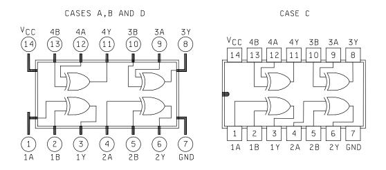
Figure 1. <u>Terminal connections (top view).</u>
