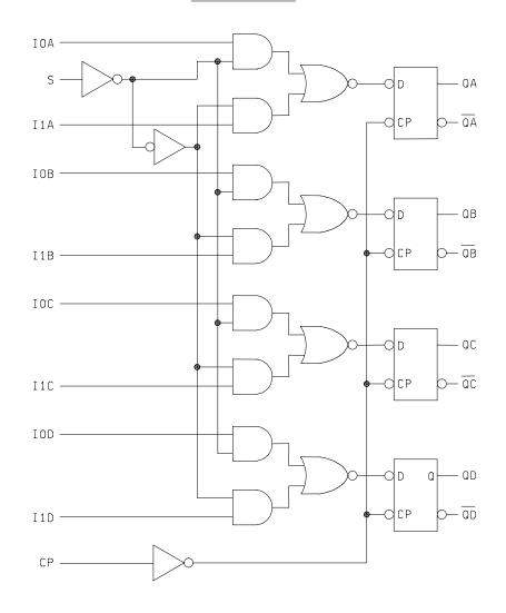
FIGURE 3. Logic diagram.
