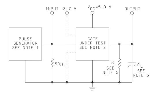
FIGURE 4. Switching test circuit.
