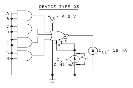
FIGURE 5. Base emitter voltage test circuit for device types 01 and 03.
