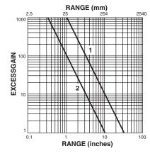
When Using Duplex Fibers for Diffuse Reflective Sensing (Gain using E51KF723 fibers, based on 90% reflective white card)
