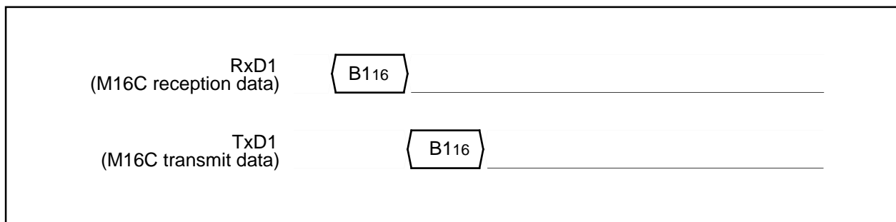
Figure 1.29.40. Timing of baud rate 19200
