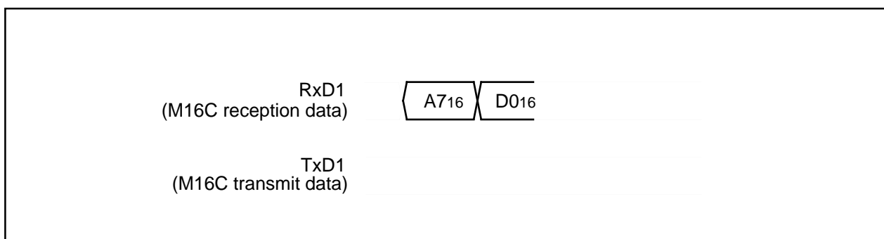
Figure 1.29.28. Timing for erasing all unlocked blocks
