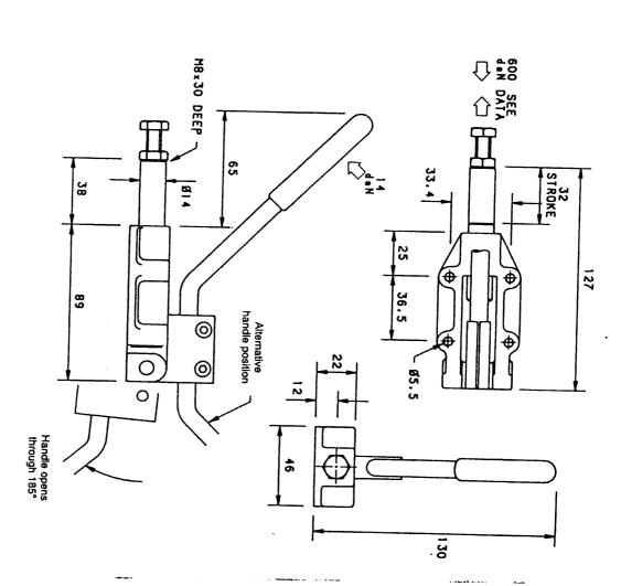
Supplied complete with: MB0840 Setscrew & nut. Nominal Holding Force: 600 daN Weight: 0.55 Kg Base: Body mounting.
