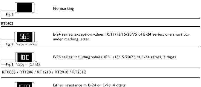
First three digits for significant figure and 4th digit for number of zeros
