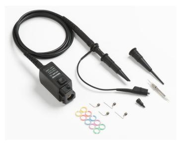
The TPP1000, TPP0500B, TPP0502 and TPP0250 models are highbandwidth, general-purpose probes from Tektronix that offer breakthrough specifications previously unrealized in this product class. Designed for use with Tektronix MDO3000, MDO4000B, MSO/DPO4000B and MSO/ DPO5000B Series oscilloscopes, these probes provide up to 1 GHz of analog bandwidth with less than 3.9 pF of capacitive loading.
