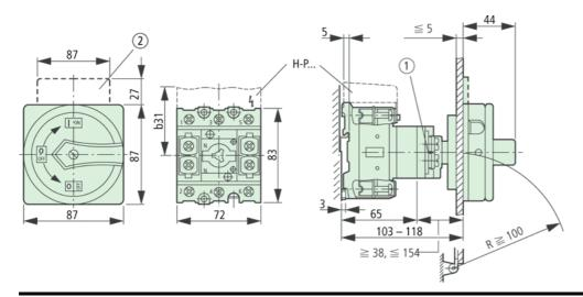
Shaft can be extended using ZVV–... + ZAV–..., max. F 4  $\times$  25 = 100 mm Not included
