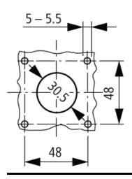
Diameter of drilled hole Door
