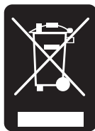
Fig. 1.4: Product labeling in accordance with EN 50419
