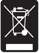
Fig. 1.4: Product labeling in accordance with EN 50419
