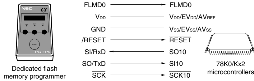
Figure 27-4. Communication with Dedicated Flash memory programmer (CSI10)
