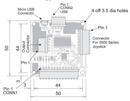
USB connection is made via either a 5 way 2.54mm pitch Molex® KK style header or a Micro USB type B socket on the board. A suitable USB cable (1.5m long) is included.
