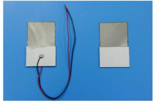
The ultrasonic vibration micro nozzle consists a piezoelectric ceramic and a metal foil, on which over thousands micro nozzles formed. Using the same principle as inkjet printer, this transducer atomizes water or liquids through a matrix of micro holes of around 7-10 µm.
