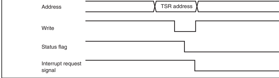
Figure 10.42 Timing for Status Flag Clearing by CPU
