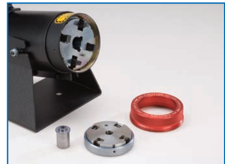
3. Pull out the Locator by hand.
