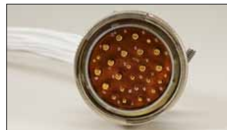
Connectors may contain several different size contacts.
