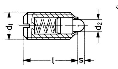
B free-cutting steel, normal spring load
