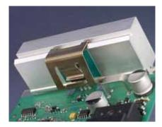
Hi-Flow 300P consists of a thermally conductive 55°C phase change compound coated on a thermally conductive polyimide film. The polyimide reinforcement makes the material easy to handle and the 55°C phase change temperature minimizes shipping and handling problems.
