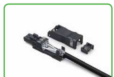
First insert the wired connector into the strain relief housing, then snap the clamp and cover.
