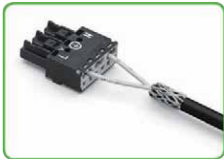
Apply the shield to the rubber cable. Strip length, outer insulation = 55 mm / 2.16 in Shield length = 10 mm / 0.39 in
