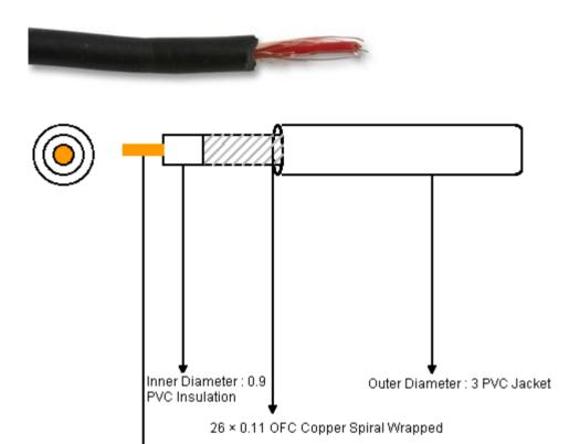
Inner Conductor: 7 × 0.11 OFC Copper Strands
