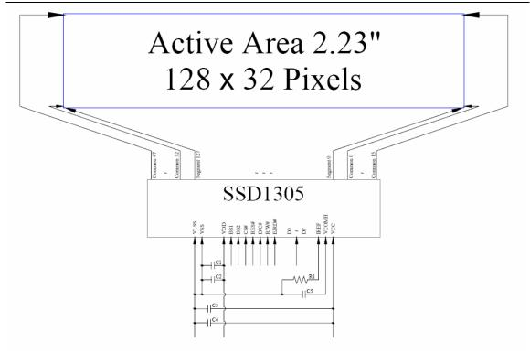
MCU Interface Selection: BS1 and BS2 Pins connected to MCU interface: D7~D0, E/RD#, R/W#, D/C#, RES# and CS#.
