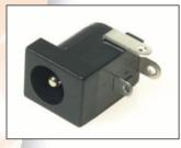
DC-10 PCB mounting pin / ring type with switch. Rated 12V / 5A. DC10A with 2.1mm dia. pin. DC10B with 2.5mm dia. pin.
