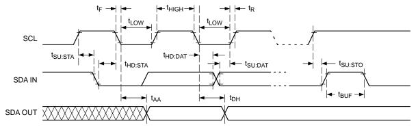
Figure 4. 2-Wire Serial Interface Timing
