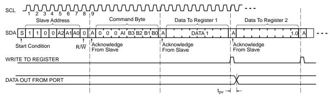
Figure 9. Write to Register Timing Diagram
