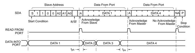
Figure 12. Read Input Port Register Timing Diagram
