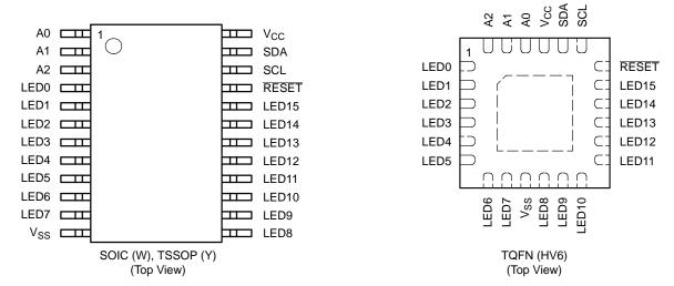
Figure 1. Pin Configurations
