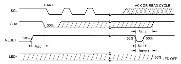
Figure 13. RESET Timing Diagram
