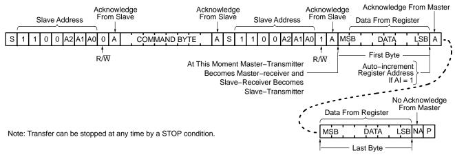
Figure 10. Read from Register Timing Diagram
