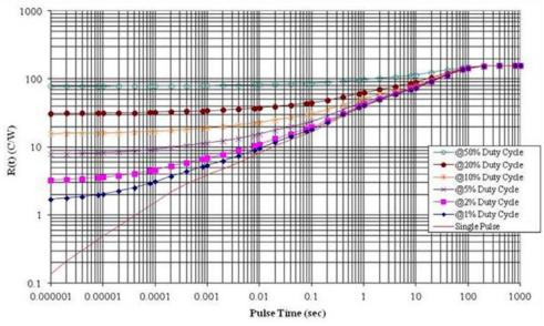
Figure 15.  $\theta_{JA}$  Transient Response Curve for TSSOP-24
