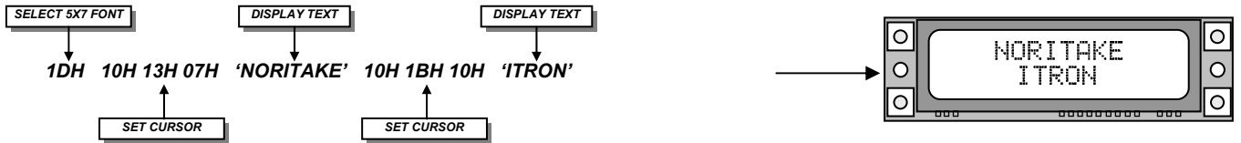
Fig1: Cursor Positioning, example of writing 2 characters from cursor position 0,7.
