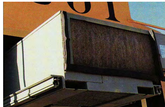
Pictured below are some custom bottom mount slides holding an air conditioner used to cool the crew compartment on a traditional style train.
