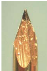
Standard Gold Coating, Contamination after 1/2 Mio contacts
