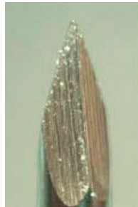
FEINMETALL „Progressive Coating“, Contamination after 1/2 Mio contacts
