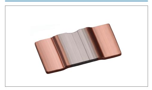
TE Connectivity is pleased to offer this Low Ohmic Surface Mount Shunt Resistor. Featuring Heavy Copper connectors, electron beam welded to a Manganin or NiCr alloy element, this resistor offers excellent long term stability and low inductance, and can be mounted using re-flow soldering techniques or welding on copper.
