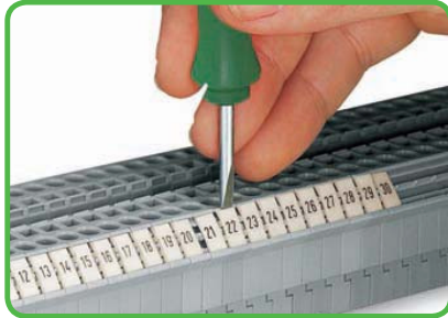
Snapping a strip into the marker slot.
