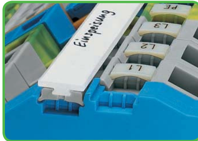
Carrier for WFB Continuous marking strip; to be secured every 10th terminal block.
