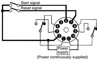
**2. Signal-ON-OFF Start/Instantaneous Operation/Time-limit Reset**
