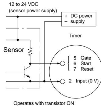
No-voltage Input Signal Levels
