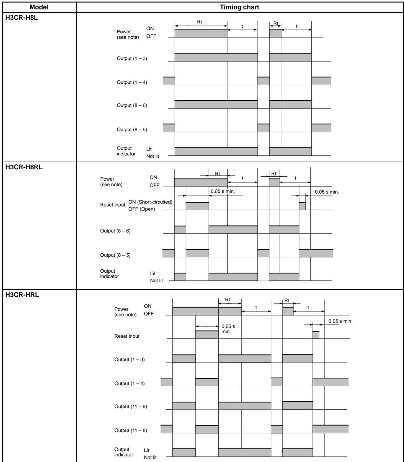
**Note:** If the power is turned ON until the set time is up, the timer will be retrigged.
