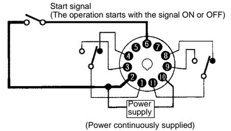
**C Mode: Signal ON/OFF-delay**
