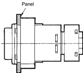
**Note:** The adaptors for two or more timers mounted in a vertical line are different in orientation from those mounted in a horizontal line.
