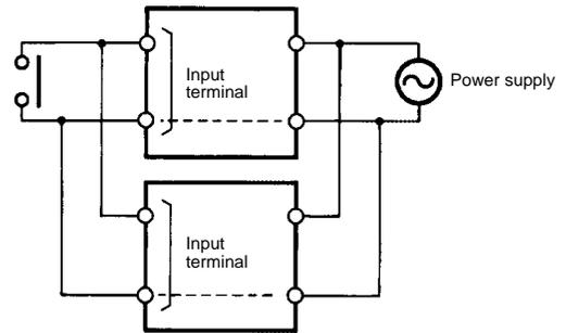
It is impossible to provide two independent power switches as shown below regardless of whether or not the Timers are different in phase.
