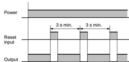
If it is required that the output be turned on repeatedly with an interval of shorter than 3 s, consider use of the H3CR-A in mode D (signal OFF-delay).
