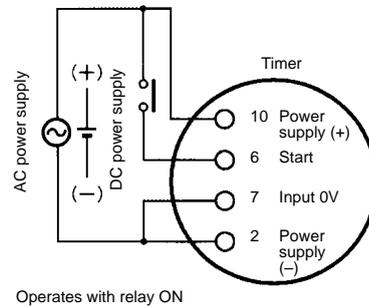
**Note:** The input circuit is isolated from the power supply circuit. Thus, an NPN transistor can be connected.
