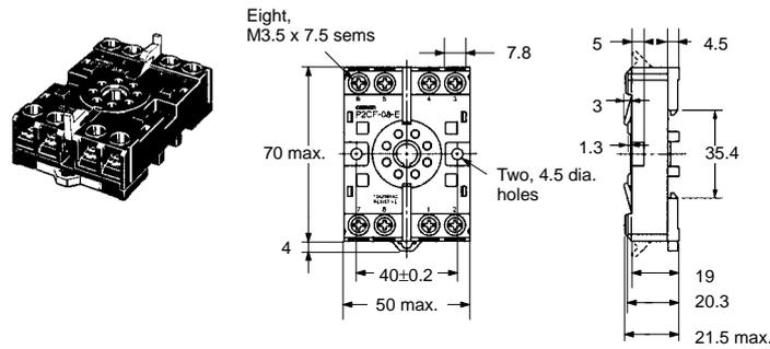
**Track Mounting/Front Connecting Socket**
