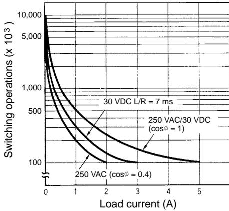
Reference: A maximum current of 0.15 A can be switched at 125 VDC ( $\cos\phi = 1$ ) and a maximum current of 0.1 A can be switched if L/R is 7 ms. In both cases, a life of 100,000 operations can be expected. The minimum applicable load is 10 mA at 5 VDC (failure level: P).
