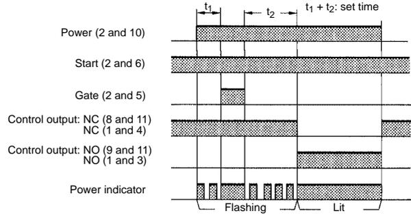
Gate signal (The operation is interrupted with the gate signal if the Timer detects an abnormal signal.)
