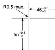
**Note:** The mounting panel thickness should be 1 to 3.2 mm.
