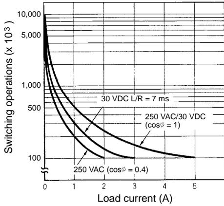
Reference: A maximum current of 0.15 A can be switched at 125 VDC (cosφ = 1) and a maximum current of 0.1 A can be switched if L/R is 7 ms. In both cases, a life of 100,000 operations can be expected. The minimum applicable load is 10 mA at 5 VDC (failure level: P).
