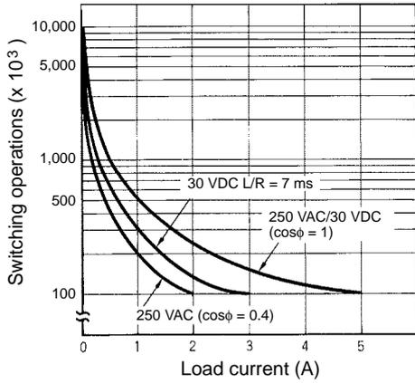
Reference: A maximum current of 0.15 A can be switched at 125 VDC (cosφ = 1) and a maximum current of 0.1 A can be switched if L/R is 7 ms. In both cases, a life of 100,000 operations can be expected. The minimum applicable load is 10 mA (100 mA for H3CR-A8E) at 5 VDC (failure level: P).
