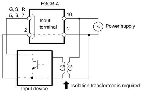
The H3CR-A□/A□S/AP's power supply terminal 2 is a common terminal for input signals to the Timer. Do not disconnect the wires on terminal 2, otherwise the internal circuitry of the Timer will be damaged.
