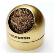
The Hakko 599B cleans soldering iron tips without water. It is made from coils of brass which is softer than the tip plating yet harder than the oxidation that forms the tip. The 599B is the ideal alternative to a wet sponge.
