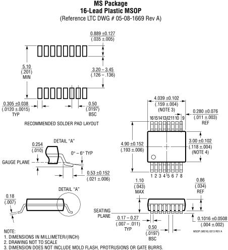
MOLD FLASH, PROTRUSIONS OR GATE BURRS SHALL NOT EXCEED 0.152mm (.006") PER SIDE
