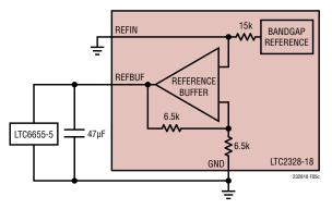
Figure 5c. Overdriving REFBUF Using the LTC6655-5
