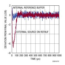
Figure 7. Transient Response of the LTC2328-18
