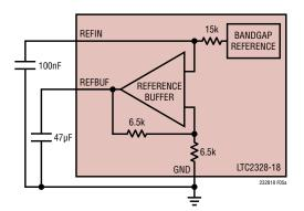
Figure 5a. LTC2328-18 Internal Reference Circuit
