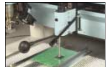
BGA placement is easy using the patented Weller ® placement templates.
