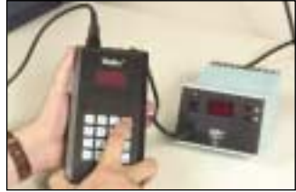
The WCB1 control module is used to set temperature lockout, set back, and °F to °C conversion.
