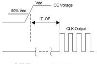
T\_OE: Time to re-enable the clock output
