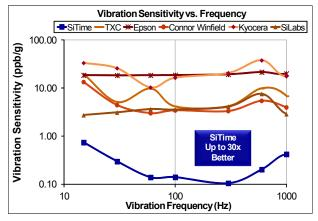
Figure 5. Vibration Robustness<sup>[5]</sup>
