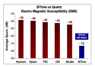
Figure 3. Electro Magnetic Susceptibility (EMS)<sup>[3]</sup>
