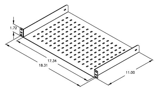
D-4455 all-in-one shelf mounts equipment on the inside or the outside of standard 19" enclosures and racks. Rugged 14-gauge steel construction.
