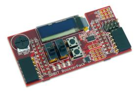
VDD\_OLED control is used to turn on/off the power to the logic of the display. The VBAT\_OLED control is used to turn on/off power to the OLED display itself. These two pins have pull-up resistors to turn off their respective power supplies when not being driven. The pins are made to be outputs and are driven low to turn on the power supplies.
